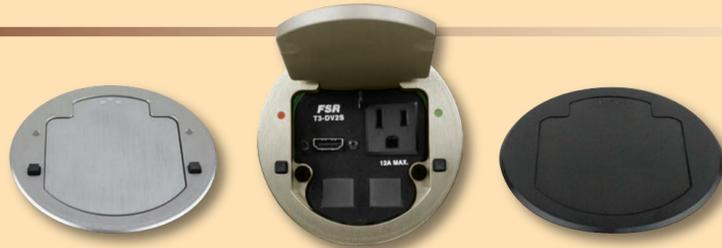
The T3-DV2S is HD ready with a bulkhead mounted HDMI connector and two keystone openings for network connectivity, FSR's snap-in USB charger and many other FSR Simple Solutions snap-in connectors. Two blanks are included with all models. For convenience, an integral AC outlet with cord is ready to power a laptop or mobile device.
